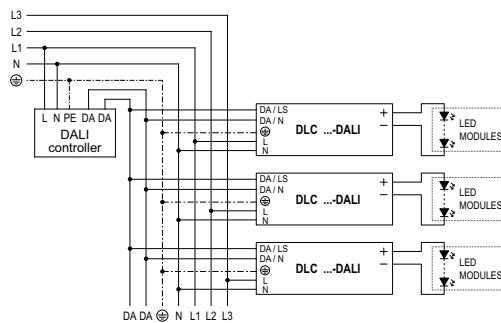
~ **Corridor function:** Dimming system that controls light level when a presence is detected by a conventional mains on/off sensor connected in DALI input. When the sensor detects a presence, light level increases up to 100%, otherwise the control gear keeps on providing 10% light level.
